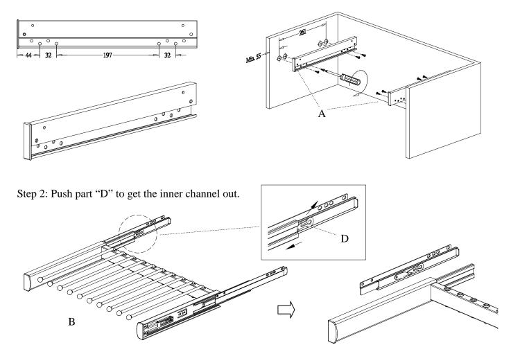
Step 3: Screw inner channel to aluminum spacer. Join outer slide together with the inner channel.
